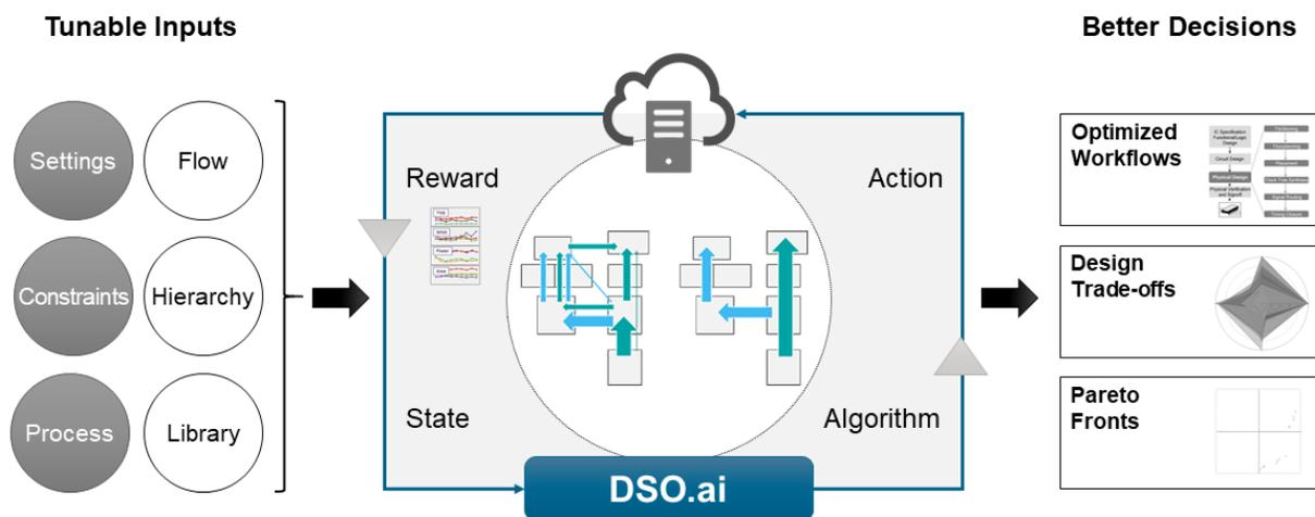
**Synopsys DSO.ai shifts the burden of optimization from the traditional reliance on manual sweeps to one that relies on large computation to autonomously identify design spaces of potential solutions.**
