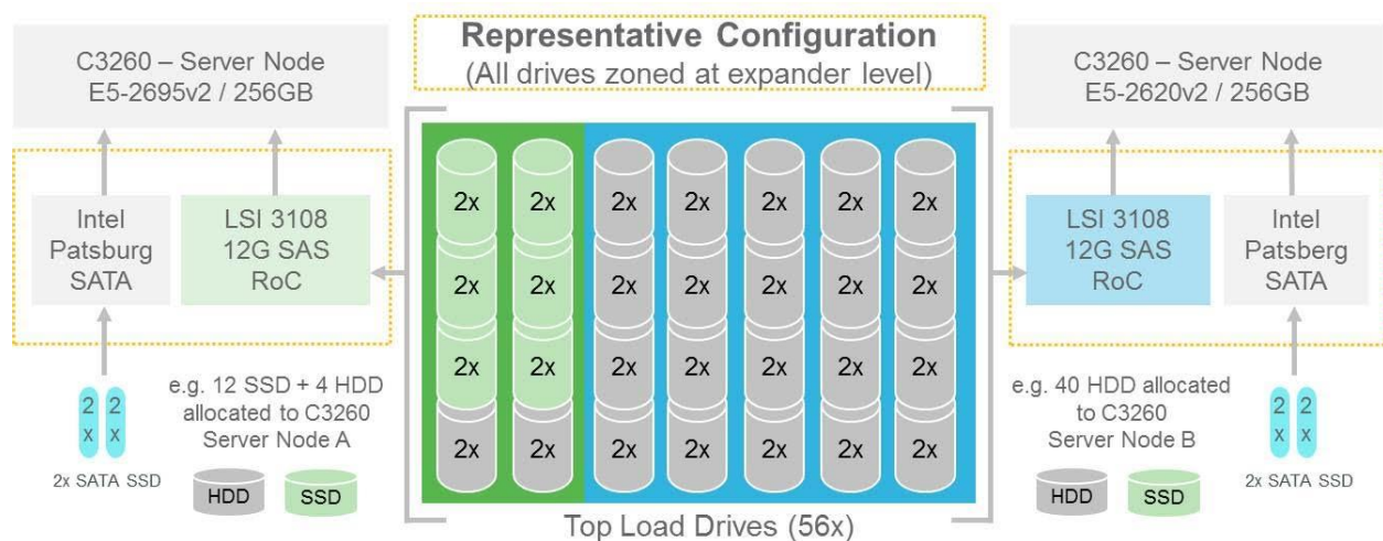
FIGURE 3: CISCO UCS C3260 DISAGGREGATED INFRASTRUCTURE
