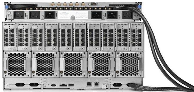
The Apollo a6000 chassis does not have an internal power source but rather relies on connections from the chassis to the HP Apollo 6000 Power Shelf which provides shared power across enclosures for efficiency and redundancy. The Apollo 6000 Power Shelf is 1.5U tall, and supports up to 6 power supplies (14.4kW or 15.9kW non-redundant or configurations that include N+1, N+N redundancy). One power shelf can support 3-4 fully loaded enclosures or up to 6 moderately provisioned chassis.
